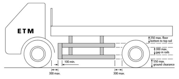
Double rail kits are suitable for vehicles not exceeding 1400mm from the undersurface of the side rave to the ground.
